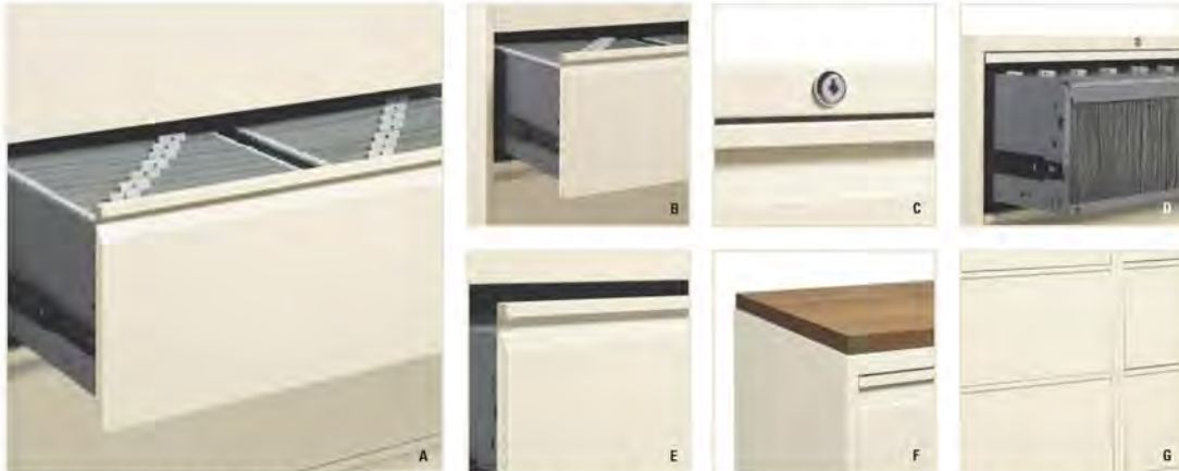
A. Front to Back filing capability. B. Full extension 3 stage ball bearing drawer suspension. C. Core removable cam locks. D. Hanging file storage in receding door openings (on 5 high models only). E. Angled recessed full pull. F. Optional lateral file tops. G. Horizontal lines – uniform and consistent providing clean, flowing look.
