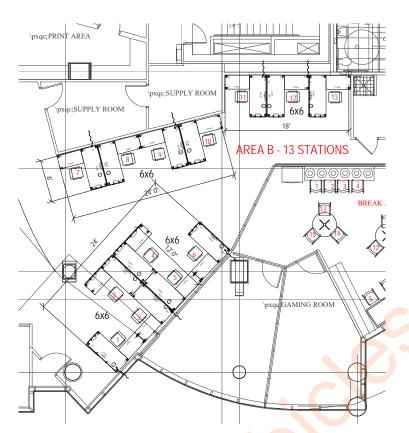
AREA B STRETCH BENCHING SYSTEM: [13] 6x6 L-SHAPE POWERED STATIONS With:
