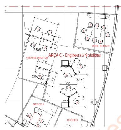
AREA C STRETCH BENCHING SYSTEM: [4] 2.5x5 STRAIGHT POWERED STATIONS With:
